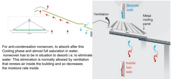
Ventilation is normally brought at ridge and bottom of slope and with additional air entrance according to building rules in force and building size.
